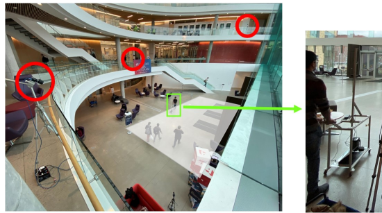
Fig. 3: Hardware setup for the TBD pedestrian dataset. Red circles indicate positions of RGB cameras. Green box shows our mobile cart with a 360 camera and stereo camera which imitate a mobile robot sensor suite. The cart is manually pushed by a researcher during recording. The white area is where trajectory labels are collected.
