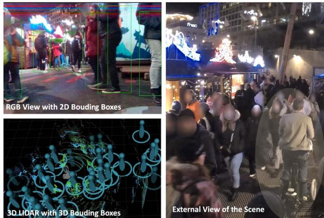
Fig. 1. Robot Qolo navigating on the crowds up to 1ppsq in density, the dataset includes annotated 3D BBx and 2D BBx on Lidar and RGBD data, respectively.
